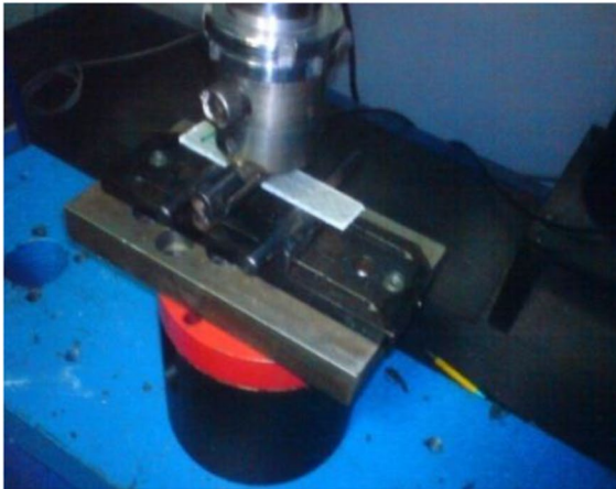
Fig. 21 Three point flexural test setup. a Top view. b Front view
